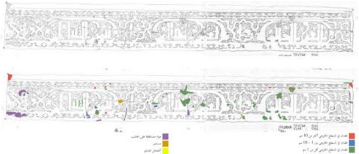
Example of the documentation and condition survey of the lower inscription frieze.
